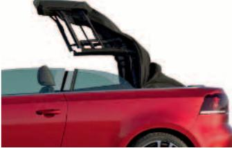
*The cloth soft top of the new VW Golf Cabriolet consists of three layers in total which render it inherently stable.*
