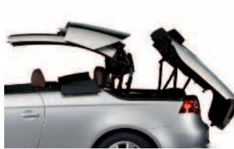
*The metal hard top of the VW Eos is the world's first convertible roof that consists of five individual roof sections.*
