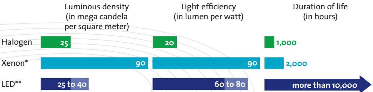
\* Values correspond to a xenon headlight with 35 watts output.
