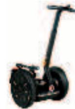
The Segway is controlled by the driver's weight: If you lean forward, backwards or to the side then the vehicle drives in that particular direction.
