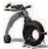
The rider of the Yikebike puts his feet down while riding and steers the electric vehicle with the handlebar behind the seat.
