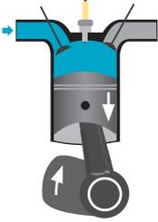
**Petrol engine:** The suction process conveys the fuel air mix into the cylinder.
