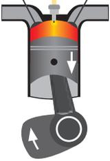
**Petrol engine:** The spark plug ignites the fuel air mix. It expands explosively and pushes the piston downwards.
