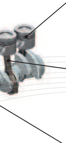
The **pistons** are pushed downwards by the pressure that results from the expansion of the fuel air mix during combustion.
