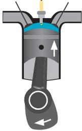
**Petrol engine:** The fuel air mix is compressed by the upward stroke of the piston and is thus heated up to 400 to 500 degrees.
