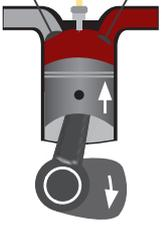
**Petrol and diesel engines:** Finally, the piston is pushed upwards again due to its connection to the crankshaft, releasing the resulting emissions.
