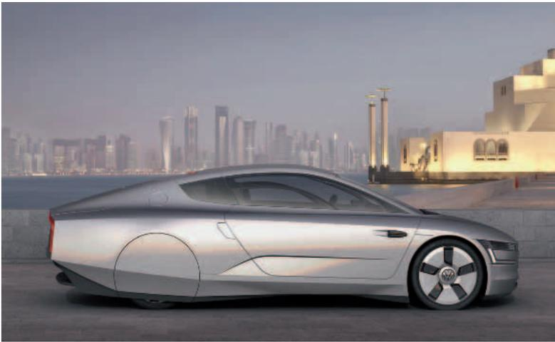
*Thanks to a combination of lightweight construction, low aerodynamic drag and a plug-in hybrid system, the Volkswagen prototype XL1 answers the question of how much the energy consumption of a car can be reduced.*
