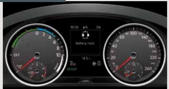
The power meter supplements the rev counter on the left side of the instrument panel. It indicates if the high-voltage battery is currently charging via recuperation or if energy is being discharged.
