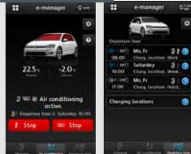
The “Volkswagen Car-Net e-remote” smartphone app can pre-set the climate control, the departure time and control battery charging. In addition, parking spaces can be located remotely and it also checks if the doors are closed. Vehicle data and statistics, such as kilometres driven, driving time and fuel consumption data are available on demand.
