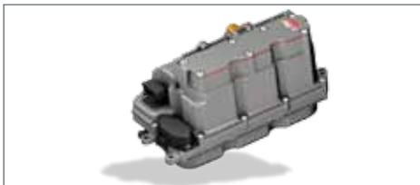
The power electronics are responsible for the conversion of electric current. To do this, it is connected to the electric motor and the battery. In electric motor mode, six high-power transistors convert the direct current of the high-voltage battery into a three-phase alternating current that powers the electric motor. In generator mode, the power electronics rectify the alternating current generated. This supplies the electrical system and charges the high-voltage battery.
