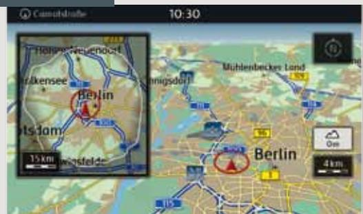
A map of the environment shows the current possible radius of action when driving purely electrically. Nearby charging stations as well as the remaining range can be displayed.
