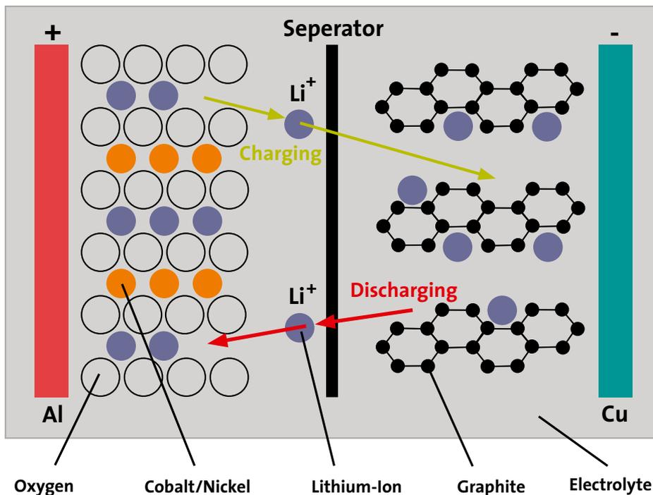
*This simple representation of a setup of a lithium-ion high-voltage battery illustrates the running processes: The lithium-ions (purple) move from the cathode (red) to the anode (blue) and accept electrons there. At the discharge process they donate electrons while moving back.*
