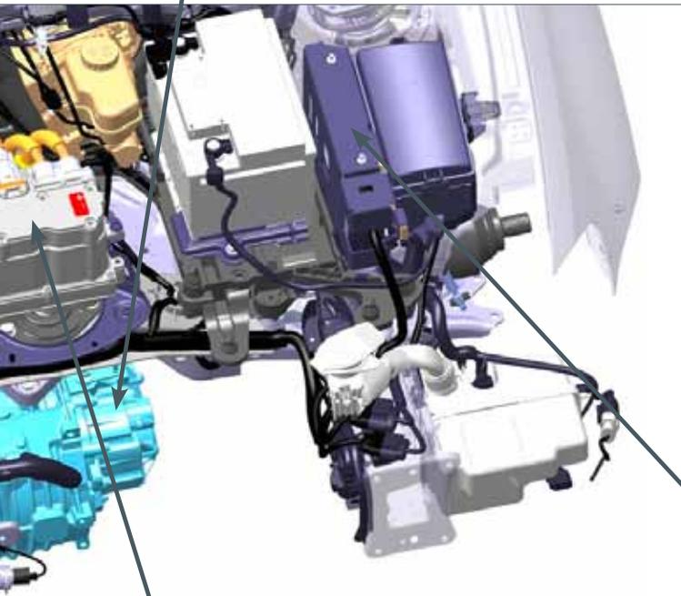
*The drive of the e-Golf is compact and light: the motor, gearbox and power electronics combined weigh only 110 kilograms.*
