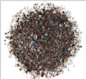
**Shredder sand** consists of glass, rust, colour particles and minuscule metal fragments which are generated during the numerous comminution processes of the VW-SiCon Process. The main objective is to reuse the shredder sand as a construction material. In order to do so many procedures have to be developed to separate sand and metal parts from each other (see Interview).
