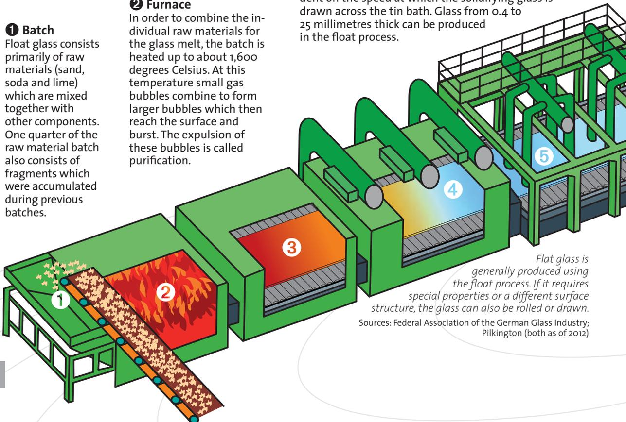
*Flat glass is generally produced using the float process. If it requires special properties or a different surface structure, the glass can also be rolled or drawn.*
